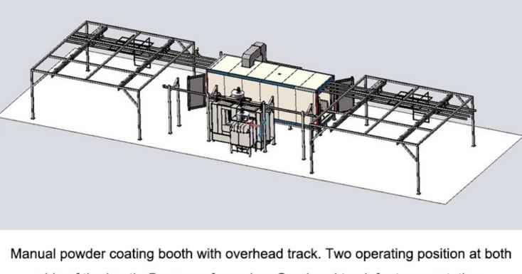
side of the booth. Box oven for curing. Overhead track for transportation. Suitable for work piece less than length 6m, width 1m, Height 2m. CUSTOMER PROVIDED PHOTOS
